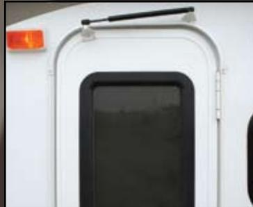
Radius exterior door with gas strut provides strength and durability compared to a square door with a plastic latch.
