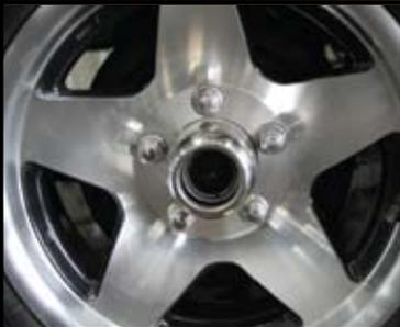
Easy lube axles make wheel maintenance easy! No need to take the whole wheel off when repackaging wheel bearings.
