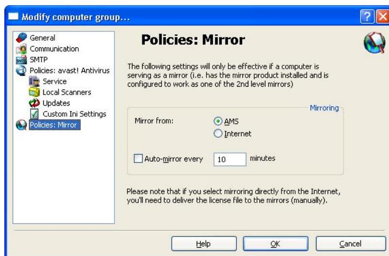
Figure 6.8. Properties of the Mirror product (the second-level mirrors)
