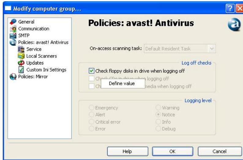
**Figure 6.1. Overriding parent group policies. The “Define value” menu is brought up by using the right mouse button.**
