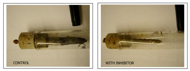
Both test tubes containing an amount of water had a steel nail pushed through the corks. One of the test tubes has the pure amine inhibitor added to the water. The nail in the control sample corroded and produced an expansive volume change as we see in corroded reinforcement. The protected nail had a layer of passivated surface corrosion form that protected it. The tip of the nail remained shiny, indicating an anodic effect.
