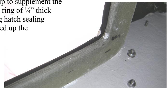
A thicker and softer rubber strip was placed on this hatch flange extension and seals well against the hatch cover. When the cover is off the seal rubber also nicely creates a raised lip to prevent water dripping off the rear deck and into the compartment. New hold down latches were added to provide seal compression along the previously unsecured front edge.
