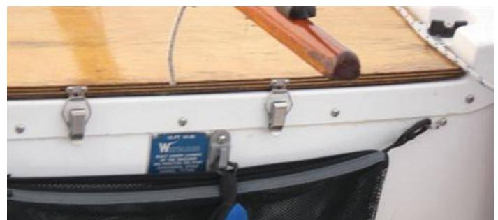
It hasn't yet been capsized tested this year, but I am far more confident the rear compartment won't end up full of water. I am still considering adding an inspection port into the wooden cover to allow quick access to smaller items when underway.
