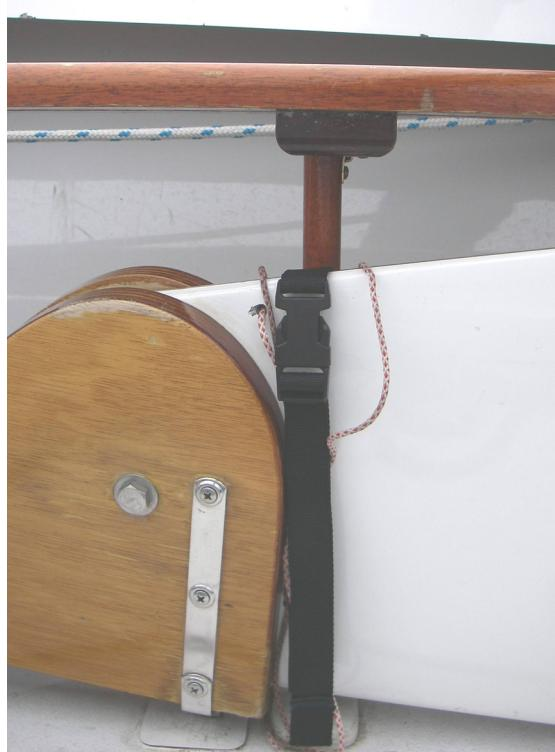
The very chunky plywood blocks originally provided for the floor seat post restraint were re-fabricated out of fibreglass pieces that now allow water to drain out and won't rot. The height was significantly reduced and these will be more comfortable to sleep on too. The lowered base did require adding a fibreglass shim piece to the post end... but that now completely keeps the wood out of any moisture.
