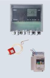
The EXHAUSTO automatic control unit EBC20 has an XTP sensor which monitors the chimney draught and supervises the fail-safe function. The unit is easy to install and commission. The display indicates the actual chimney draught as well as the value preset during commissioning, and the unit provides a variety of variable settings for the control of the system.
