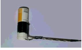
The NTC is quite robust and it does not matter if it gets a bit humid as long as it can dry again. Use a up-side down mounted tablet tube which you leave open at the bottom. This way water will be able to get out again.
