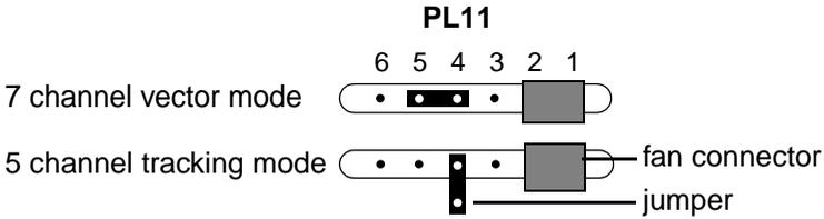
The DMX mode is set with a jumper on the circuit board inside the unit. *The factory default is tracking mode.* Follow the procedure below to change the mode.
