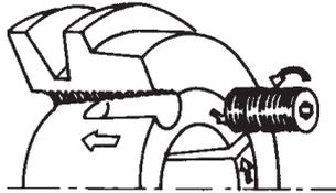
Clean and degrease all polished surfaces, adjust the hub in the pulley, level with this, positioning is correctly.
