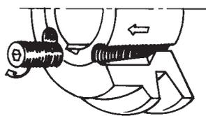
Remove the 2 screws, place one of them in the threaded extraction hole and screw completely. The hub and the pulley are thus separated one from the other.
