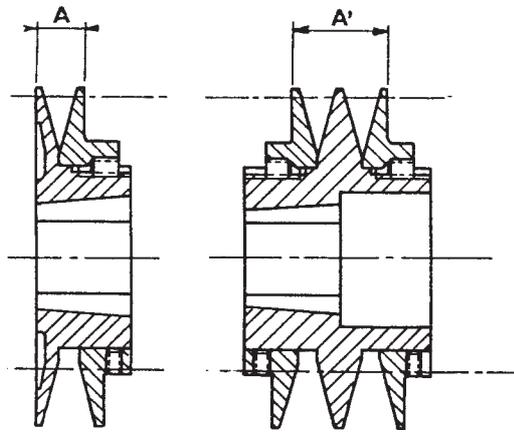
Adjustment during operation : Proceed as shown above (same as 4 to 7), taking care first to loosen screw No. 2 and to fully slacken the drive belt.
