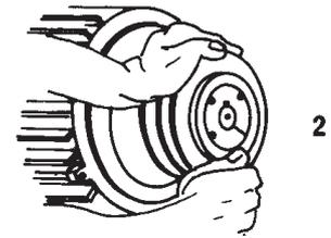
Put the pulley and its hub into place on the shaft, line them up and tighten the screws regularly and completely.
