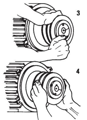
Withdraw the hub and the pulley thus feed, by and without damaging the machine.
