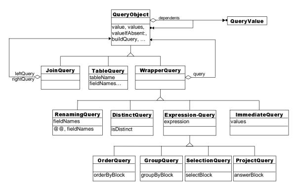
Figure 22 - Object diagram for QueryObject
