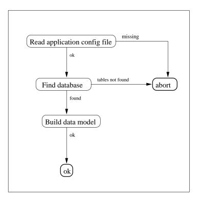
Figure 35 - Application Setup
