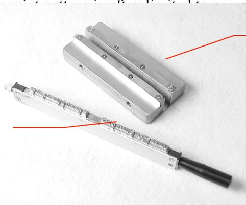
1. Insert the Adapter Sleeve into the Heater Platen and lock it by flipping the Butterfly Clips on the side of the Heater Platen.
