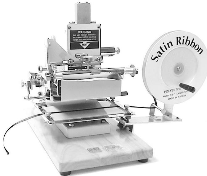
13. Make a few test prints, and make any necessary adjustment to the ribbon guide until the impression prints in the center of the ribbon. Adjust the temperature as necessary.
