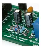
STEP 4: Solder the Voltage Regulator. Note the orientation of where the "flat side" is facing.
