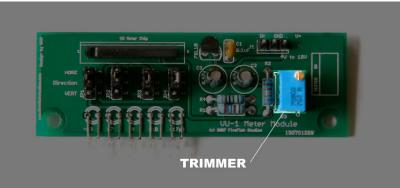
The VU Meter Kit features a 25-turn trimmer potentiometer. This is used for calibrating your VU Meter. (More on this later.)
