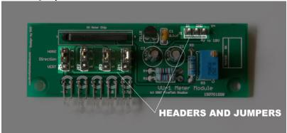
The VU Meter Kit can be installed either horizontally or vertically. Normally,  $\overline{VU}$  Meter movement go from LEFT  $\rightarrow$  RIGHT or BOTTOM  $\rightarrow$  TOP direction.
