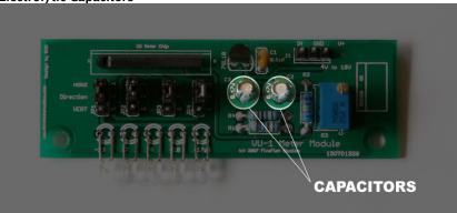
Electrolytic capacitors are cylindrical in construction. Unlike ceramic capacitors, electrolytic capacitors USUALLY/MOSTLY have polarity. One side is marked with the (-) sign, also called the cathode, or negative side.
