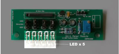
LEDs are a special kind of diode that lights up when current goes through it. We're using low-current, high efficiency LEDs for the VU Meter Kit. These are crystal clear when OFF, and bright RED when turned ON. Insert the LEDs with the longer legs on the left side, looking at the VU Meter PCB from the front.
