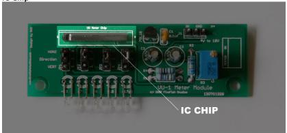
The IC chip used in the VU Meter Kit is a 9-lead SIP (Single Inline Package). One side of the chip will have a V notch. This designates where pin #1 is located. Install the IC Chip with pin #1 (V notch) on the left side of the board (looking at the VU Meter PCB from the front view.)
