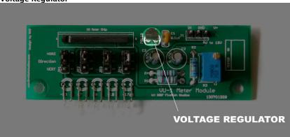
The VU Meter Kit uses an on-board voltage regulator, limiting the supplied DC voltage to the VU Meter chip to +18V. This means, you can connect this VU Meter Kit to power supply greater than +18V, for example: +24V or higher. I would suggest though that keep the input voltage to the VU Meter Kit under +25V.
