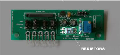
Resistors provide resistance, and are measured in OHMS, the unit of resistance.
