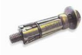
used for heavier loads. A hole of the same diameter is drilled and the bolt is inserted, just as in the case of the plastic sleeves above. However, when the bolt is tightened, after first attaching whatever you want to fix to the wall, the end of the bolt expands and anchors it firmly in the hole you have drilled. These anchors are excellent for use in solid concrete walls.
