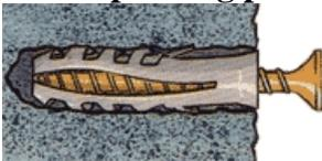
the cheapest and easiest to install of all the solid wall (*murs à matériaux pleins*) anchors. A hole of the same diameter as the sleeve is drilled into the wall, after which a screw, a normal wood screw will do, is used to attach your item to the wall. Only for fairly light loads. These non-expanding sleeves should not be used on hollow walls since they can be pulled out of drywall fairly easily.
