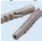
— by far the most commonly used and easiest to install. Simply drill a pilot hole of the proper dimension, insert the sleeve, often with the help of a hammer, and the action of screwing in the accompanying screw causes the anchor to expand or to deform inside the hollow space. These plastic anchors can be used for most light loads, and there is an amazing variety of sizes, shapes, and systems.
