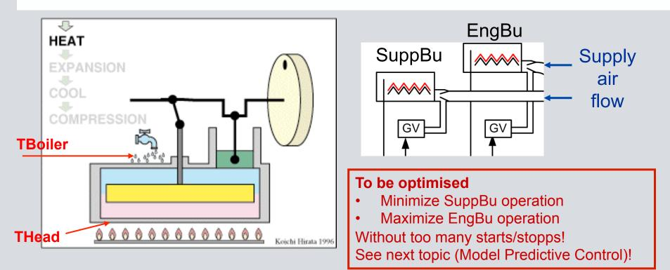
Stirling Engine (6kWth, 1kWel), Supp Burner (10..30kW)
